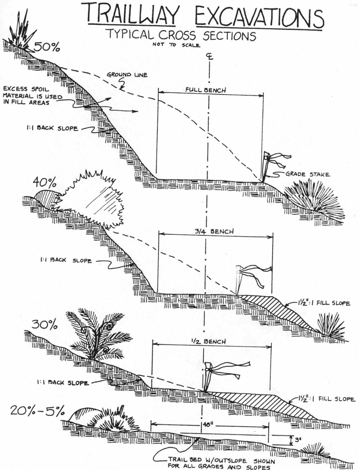
NOTE: AMOUNT OF BENCH VARIES LINEARLY W/% OF SIDE SLOPE. ALL GRADE STAKES INDICATE GRADE AT MINERAL SOIL. ALL FILL TO BE MINERAL SOIL W/NO VEGETATION DEBRIS.
